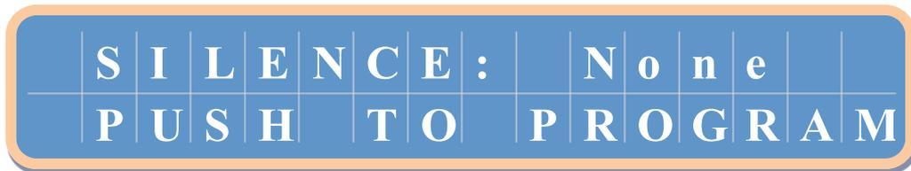
Turn encoder knob to select desired value of audio good. Move cursor to YES selection and press to confirm. New data is stored as usual
