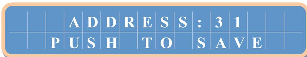
Turn the encoder knob and a specific 2-digit address can be set and saved in memory. The usual confirmation and storing procedure. The correct address for stand-alone use is “00”. When the TCP/IP optional telemetry interface is mounted, the right address is “31”.
