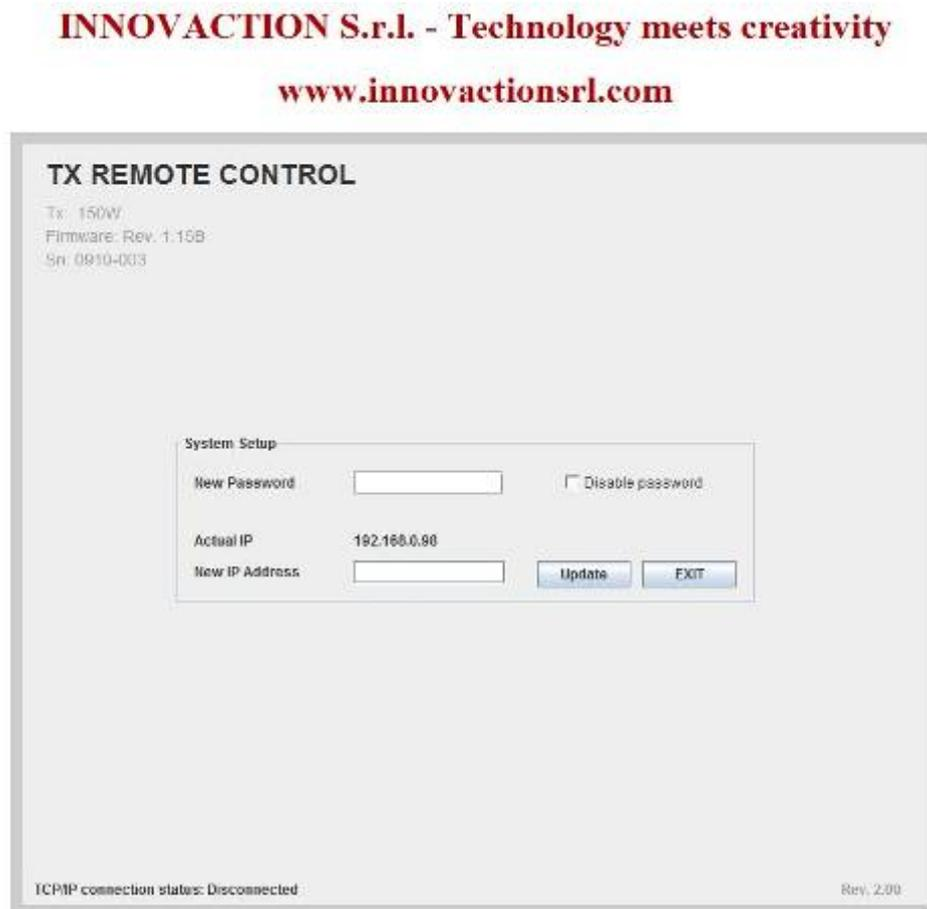
**FIG. 5 – Set-up window**
