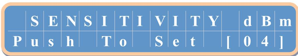
Press encoder knob and the following slide is shown
