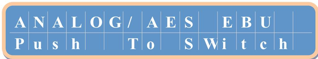
press encoder knob to select between the analog or optional digital (AES/EBU) audio input
