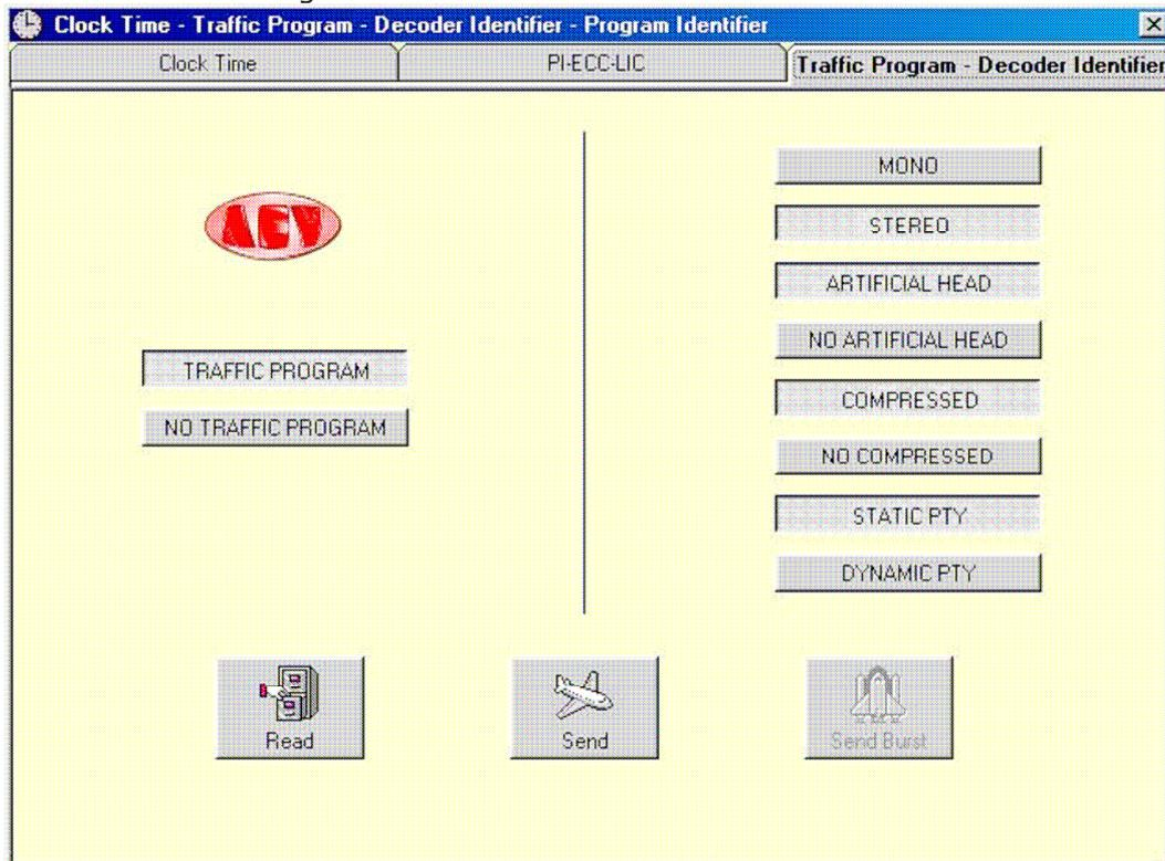
The TP option can be selected on the left side. The options relative to the type of transmission are available on the right side. Once the choices have been made, send the update to the coder using the Send push button. Use the Read push button to read
