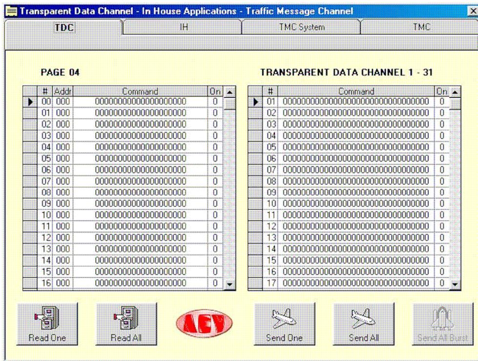
100 remote controls are available for the **Transparent Data Channel**, whereas 31 remote controls are available for the Channels from 1 to 31. As usual, the Send and Read push buttons are used for the usual functions.
