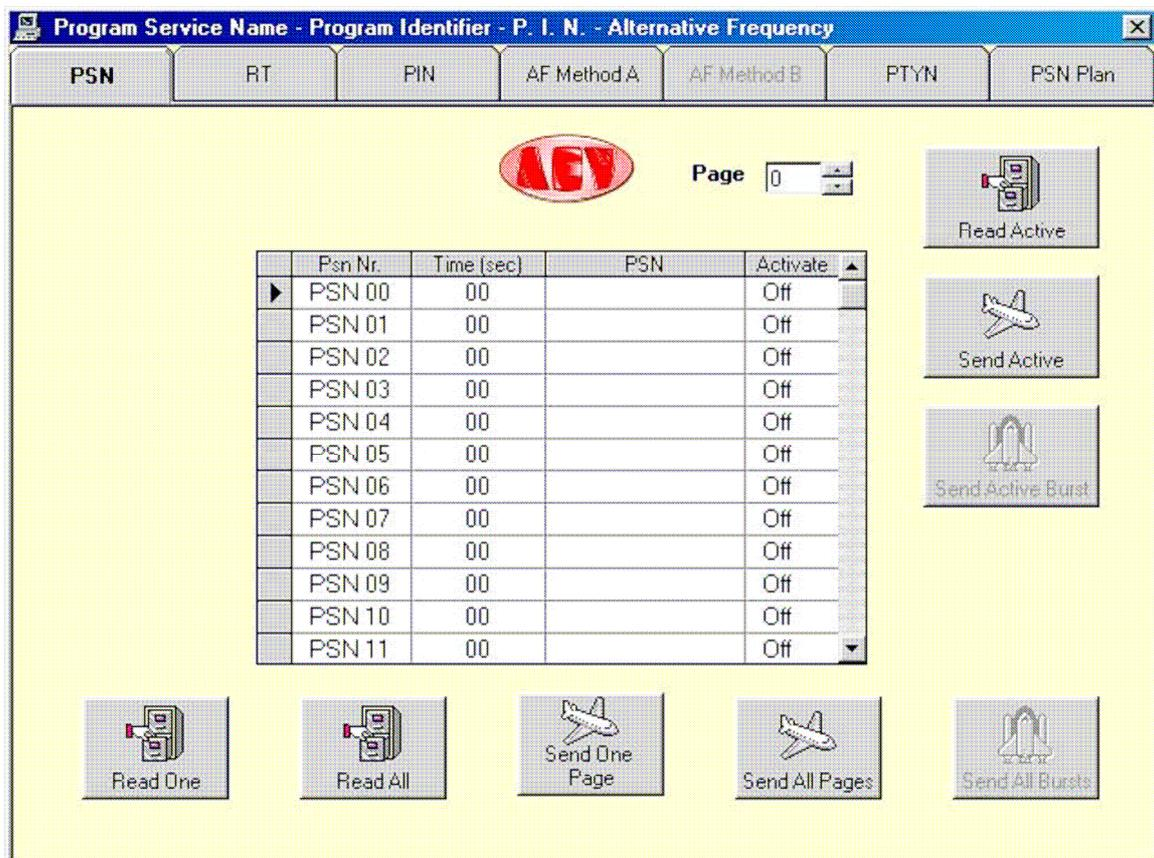
Up to 50 PSN's can be programmed. Programming is quite simple. Enter the **Time (sec)** (transmission time in seconds) of each PSN (it is advisable to enter a time of less than 3 sec). Edit the PSN, which may have a length of 8 characters, including spaces. Finally enable the PSN by double clicking on the **Activate** box of this PSN.
