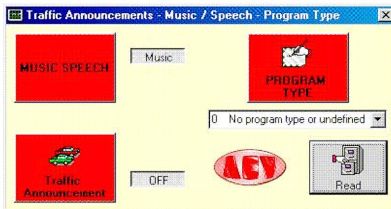
.Press any one of the red push buttons to immediately transmit the functions in use to the coder, with the exception of Program Type. To do this, make the selection using the combo box and then press the relative push button. The Read option is enabled only in "via satellite" mode.
