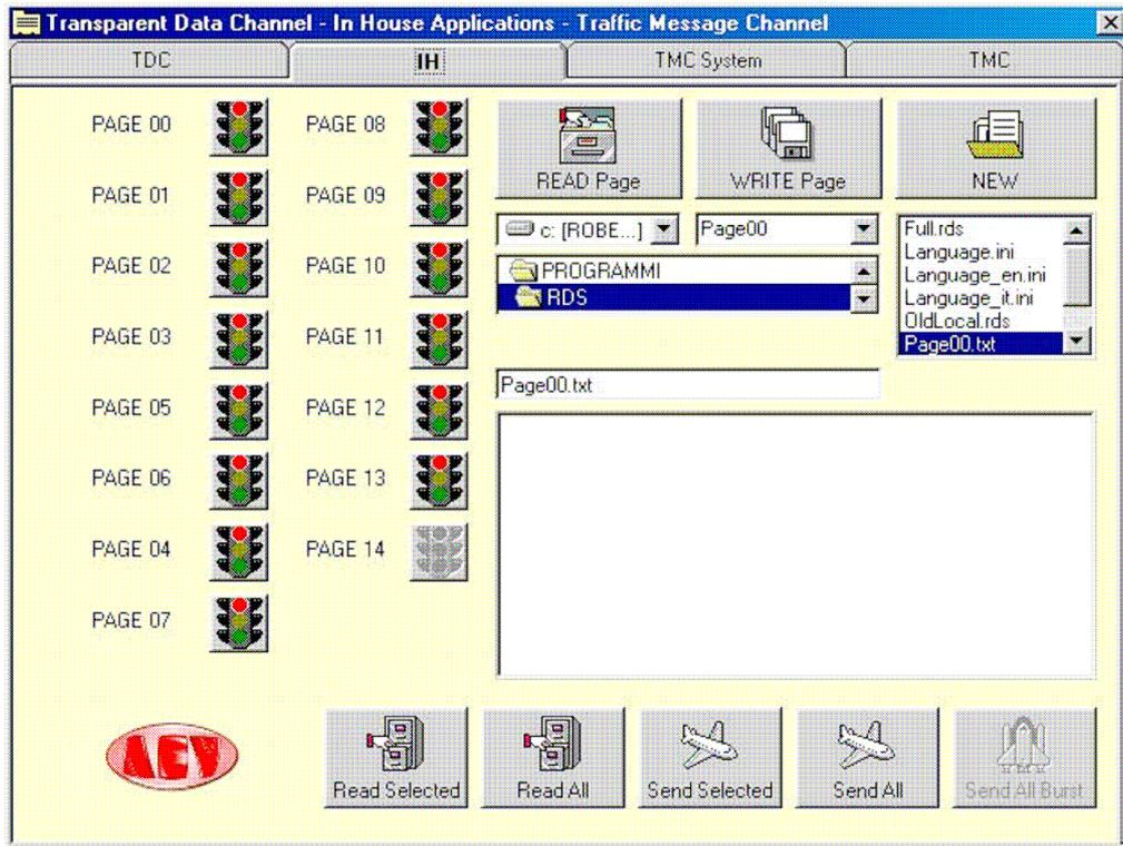
The pages available are pointed out by the lighting up of the relative traffic light. To modify a page, retrieve it using the combo box. From the editing window, make the desired modifications and then save the page using the Write Page push button or send it using the Send push buttons. A special decoder is required for this application too.
