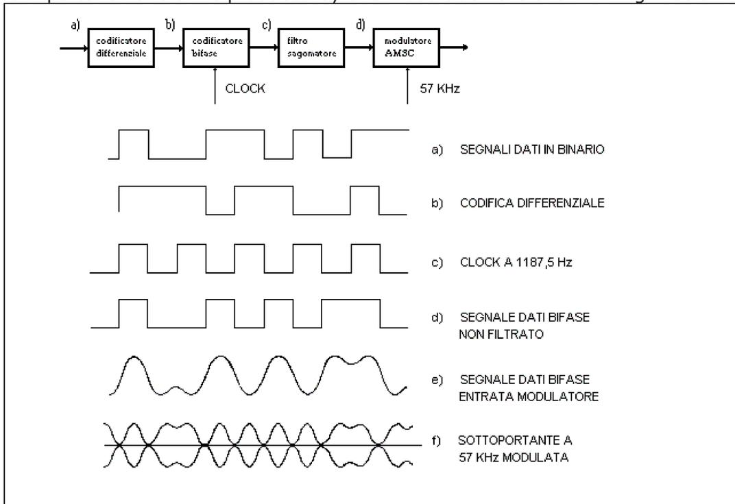
To avoid phase ambiguity on recovering the 57 KHz subcarrier, in the case of coherent demodulation, the binary data signal undergoes differential encoding prior to biphase encoding.
