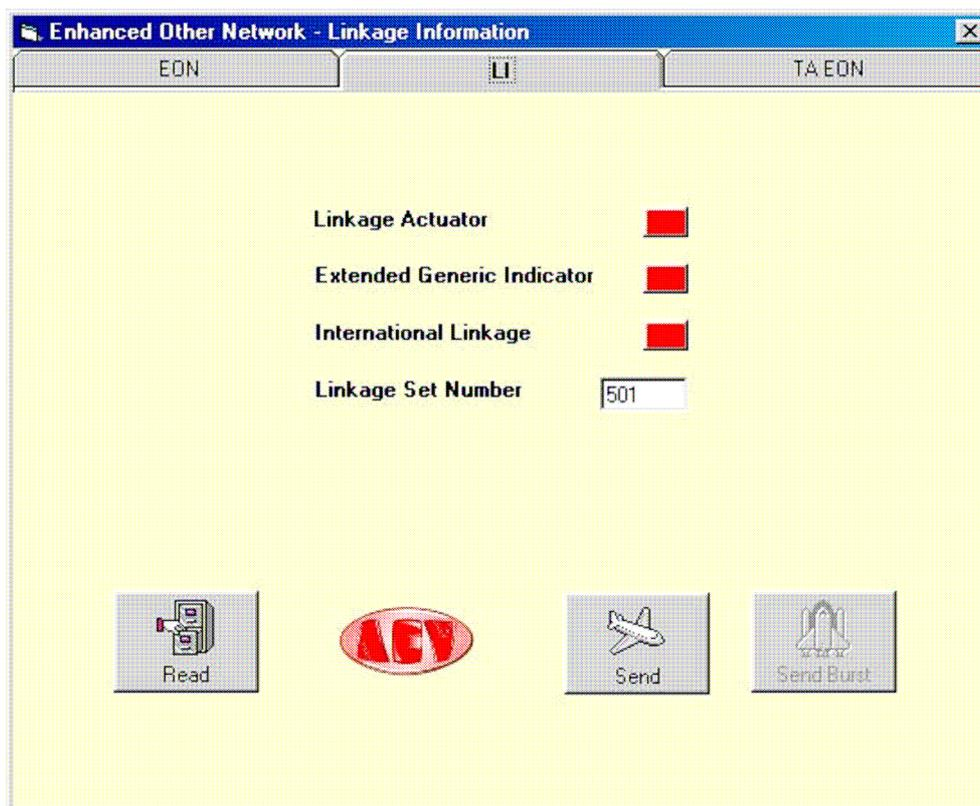
From the Linkage Information board, some parameters relative to the network transmission can be attributed. In particular using the Linkage Actuator push button, the network connection activation command is sent, the Extended Generic Indicator, which is a command not yet used, the International Linkage, which establishes whether the connection in use is of the national or international type and finally the Linkage Set Number which is the connection code.
