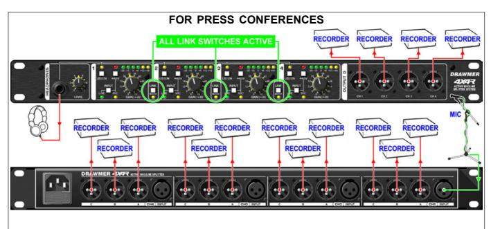
With all the link switches active, one input can be sent to all sixteen outputs - to be used in a press conference, for instance, so that all parties can have a direct feed. In such cases the output level, +48v, mic/line etc. is controlled by the CH1 parameters.
